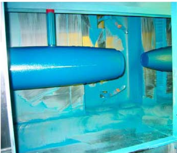
The finishing line powder coats the bombs with government-specified sky blue.
