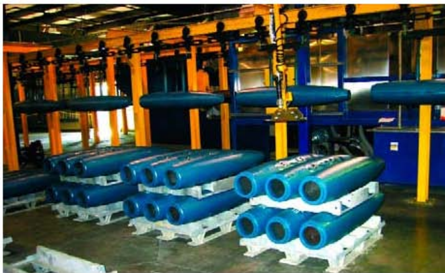
Allied Mechanical Wisconsin makes these practice bombs from cast-ductile iron. As a result they can be reused.
