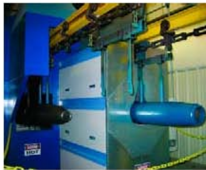
An infrared booster oven and convection oven combination cures the finish on these massive missiles.
