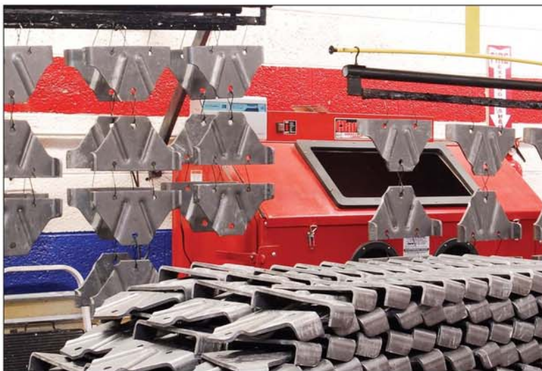
Bridgeport Powder Works treats thousands of parts, such as those seen here, using a one-step organic phosphating process.
