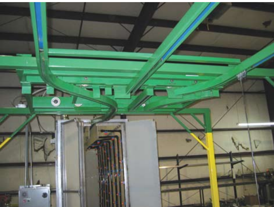
A single track enters the system; here three tracks exit headed for the oven, which can be drying a set of pretreated parts and also be curing a set of powder coated parts.
