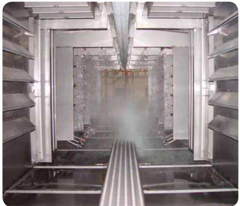
A part is treated for 60 to 90 seconds in the liquid and is then removed, dripped/blown off and dried, and is ready to be painted.
