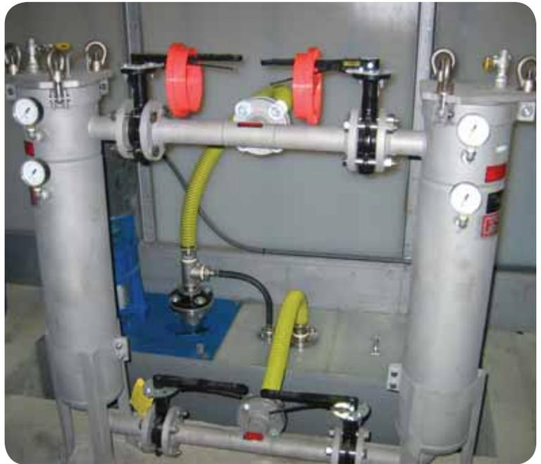
The fines that are removed from the parts at the beginning of the one-minute treatment time are separated from the bath by a bag filtration system.
